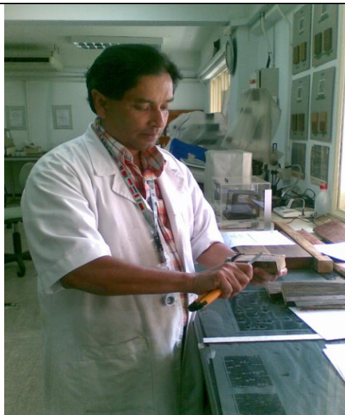
Figure 2. Cutting the wood with the knife nearly parallel with the end surface
