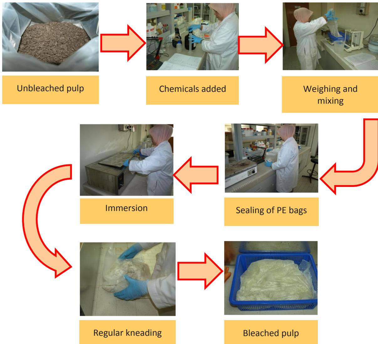
**Figure 3** Bleaching process of cellulose
