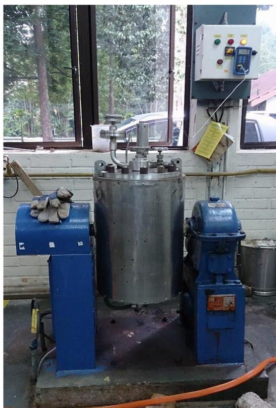
**Figure 2** Pulping in 16L rotary digester
