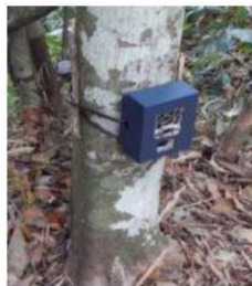
Camera trap set approximately 35-40 cm from ground surface using Phyton cable
