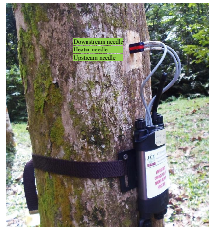
Figure 2 The sensors inserted to the tree consist of downstream, heater, and upstream needles
