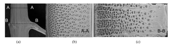
**Figure 3** Comparison between internode and node of culm; (a) radial section, (b) cross-section of internode A–A and (c) cross-section of node B–B
