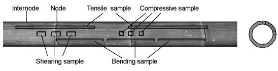
Figure 1 Testing samples produced from bamboo culm
