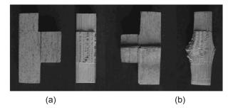
**Figure 5** Shear failure for culm (a) without node and (b) with node
