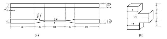
Figure 2 Dimensions of (a) tensile and (b) shear test samples (parameters are in mm)
