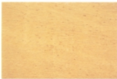
Figure 1. Irregular grain - grain that is not straight because of the abnormal structure of the wood
