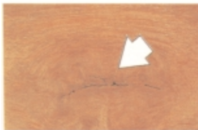
Figure 4. Dead knot (non-adhering knot) - knothaving fibres intergrown with those of the surrounding wood to the extent of approximately 75% and 25% of its cross-sectional perimeter
