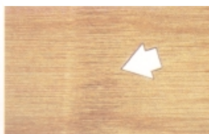
Figure 19. Sander burn - burnt mark on the outer ply caused by excessive friction during sanding
