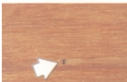
Figure 9. Worm hole (borer hole, shot hole, grub hole) - hole or tunnel or channel caused by a wood borer.
