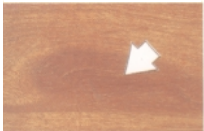
Figure 7. Included phloem - strands or zones of abnormal and often very hard tissue occurring in long or short concentric arcs in some timbers, caused by abnormal development of the cambium
