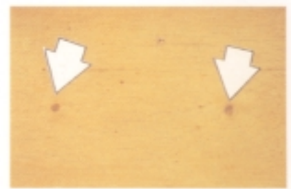
Figure 3. Pin knot - intergrown knot of not more than 3 mm in diameter
