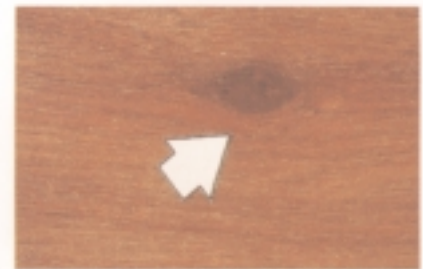
Figure 5. Sound knot - knot free from rot, solid across its face and at least as hard as the surrounding wood
