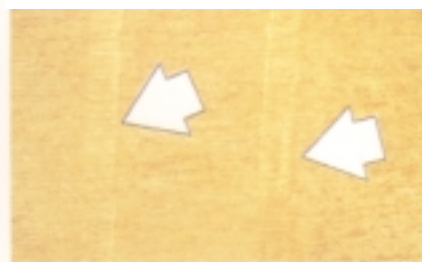
Figure 17. Chain mark - local depression on the outer ply caused by the conveyor chain
