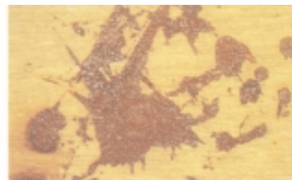
Figure 18. Glue smear - blemish that has been caused by glue splashed on the surface of veneer
