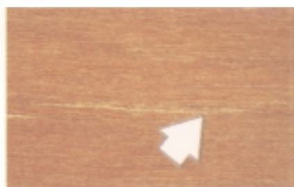
Figure 15. Split - separation of the fibres along the grain extending through the thickness of the veneer
