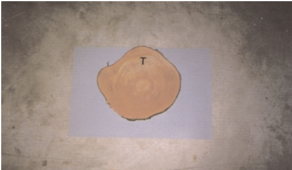
Figure 2. A disc from the stem of a rubber tree (the light-coloured zones indicate the presence of tension wood) (T)
