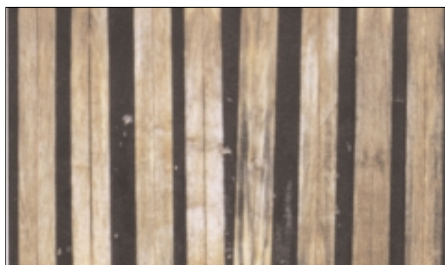
Figure 5. Typical anti-sapstain field test showing rubberwood "control" boards (without preservative) with severe sapstain
