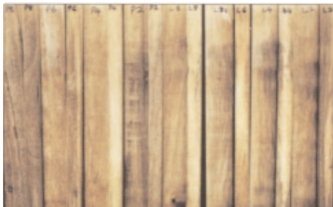
Figure 6. Typical anti-sapstain field test showing rubberwood boards treated with the reference preservative (2% NaPCP/2% borax) mixture
