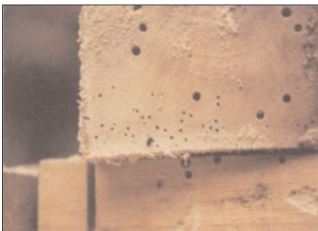
Figure 5. The smaller holes are exit holes of Minthea while the larger ones are that of the powder-post beetle, Heterobostrychus aequalis
