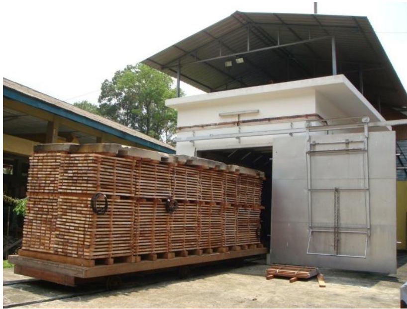
Figure 1 The prototype of high temperature drying system in FRIM campus
