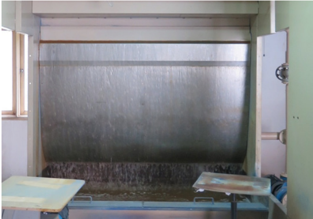
Figure 3 Water tank is covered with zinc or aluminium to protect from corrosion
