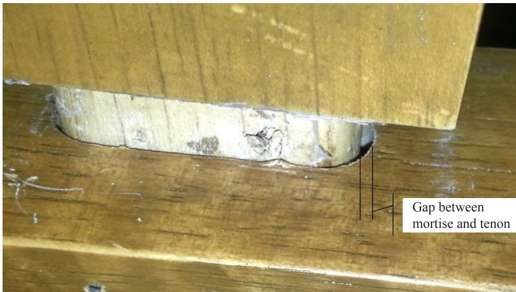
Figure 6 A considerably large gap between mortise and tenon is observed from a detached joint
