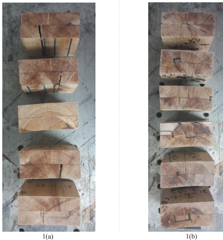
Figure 1(a) & (b) (a) Some of the test pieces that had undergone vacuum pressure test. (b) Test pieces that had undergone boiling water soak test. Pen marks indicate the length of delamination along the glue line. The photos indicate extensive checks and cracks around the pith instead of delamination.
