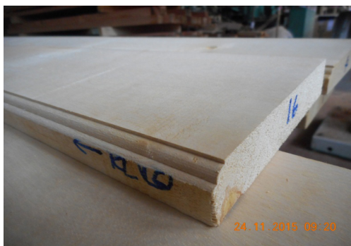
Figure 7 Wood moulded using selected profile
