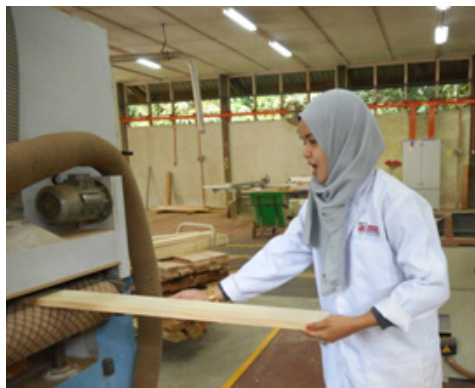
Figure 5 Sanding using 60 and 180 grit
