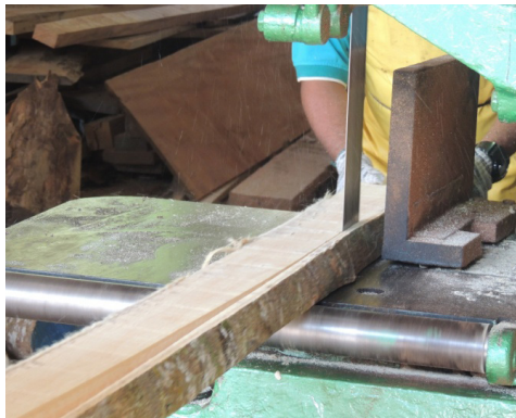
Figure 3 Sawing in green condition
