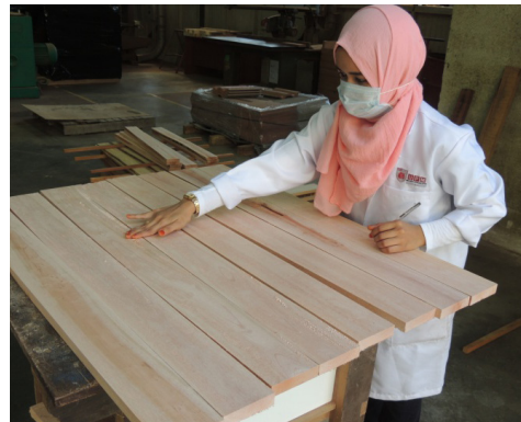
Figure 4 Surface observation after planing
