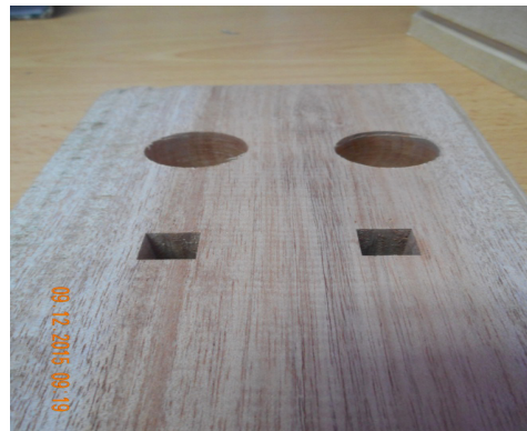
Figure 6 Bored (top) and mortised (bottom) wood
