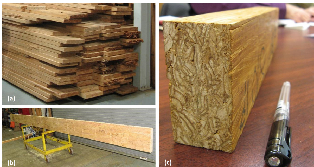
Figure 1 a) Stack of scrimber billets made at Timtek Pilot Plant; b) a 20-feet long scrimber billet from oil palm trunk; c) close-up of scrimber from Southern Yellow Pine
