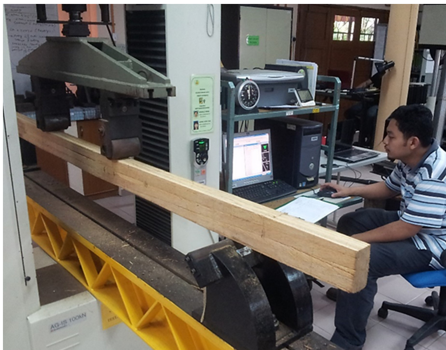
Figure 6 A 2x4 MYScrim-OPT in 4-point bending test
