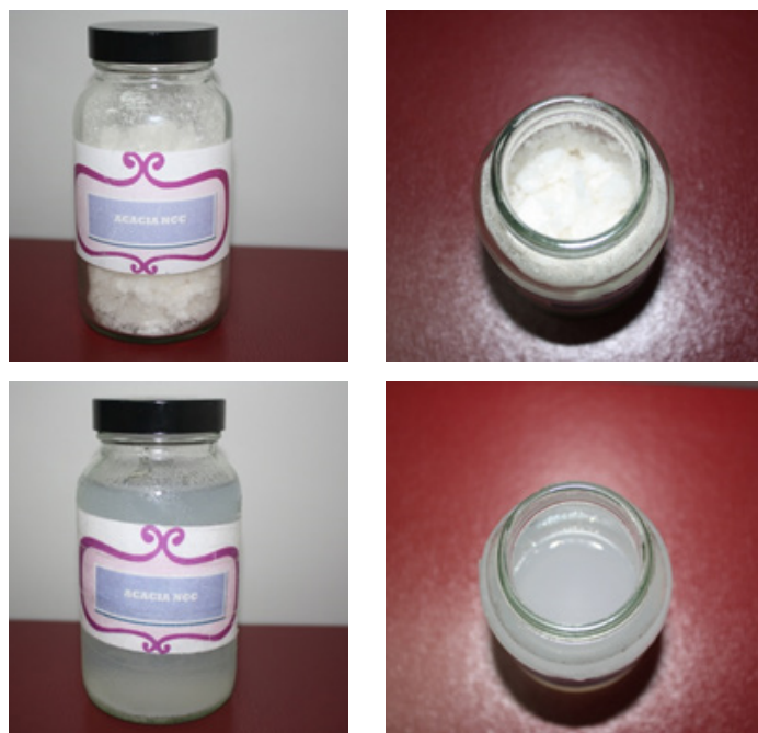
Figure 1 Nanocellulose produced from acacia wood pulp in the form of powder and suspension
