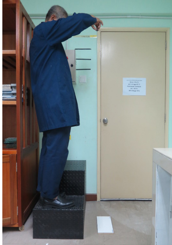
Figure 10 Steel ball dropped from 2 m heights
