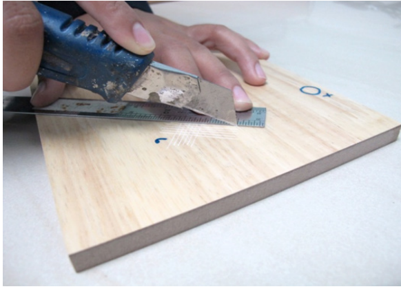
Figure 1 Cross cut test conducted based on BS EN ISO 2409:2013
