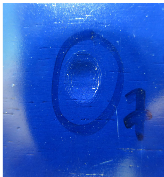
Figure 11 Effect of ball impact test on the test panel
