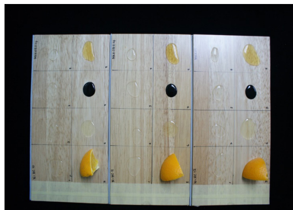
Figure 14 Household chemical are placed on the finished surface and left for 16 hours
