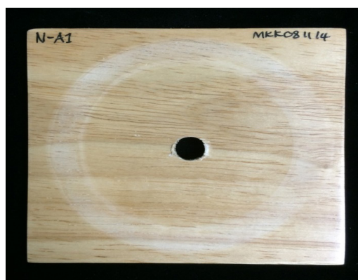
Figure 9 Effect of abrasion test after 2000 cycles
