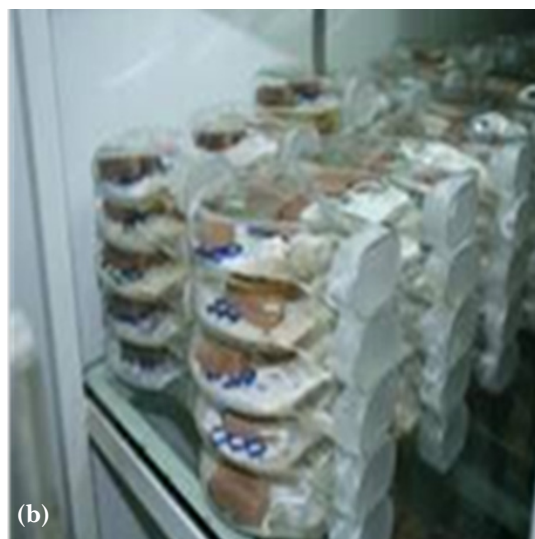
Figure 3 Laboratory decay fungi test (BS EN350-1: 1994) where (a) 3% malt extract agar containing white rot fungi, Coriolus versicolor (CV) in Kolle flask and (b) timber samples were placed into Kolle flask containing 3% malt extract agar inoculated with CV
