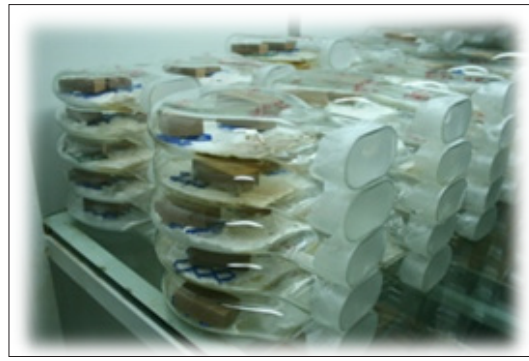
(e) Specimens tested according to BS EN 350-1: 1994
