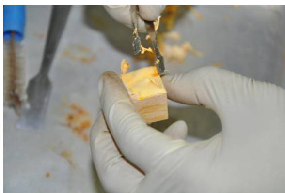
Figure 4 Removal of mycelium of CV from timber samples after 16 weeks of incubating with Coriolus versicolor (CV)
