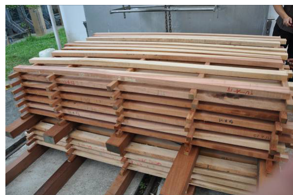
(c) Kiln drying process to achieve 12% moisture content
