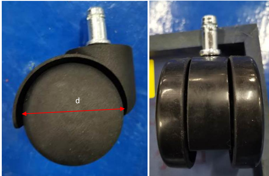
Figure 2 50-mm (left) and 60-mm (right) diameter (d) wheels made of nylon plastics
