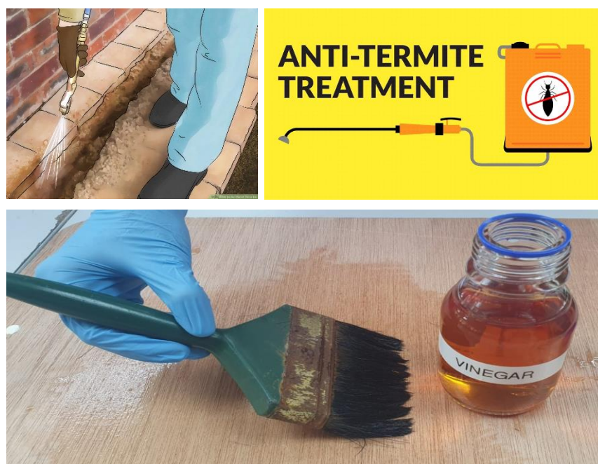
Figure 8 Wood vinegar as natural wood preservative and anti-termite application
