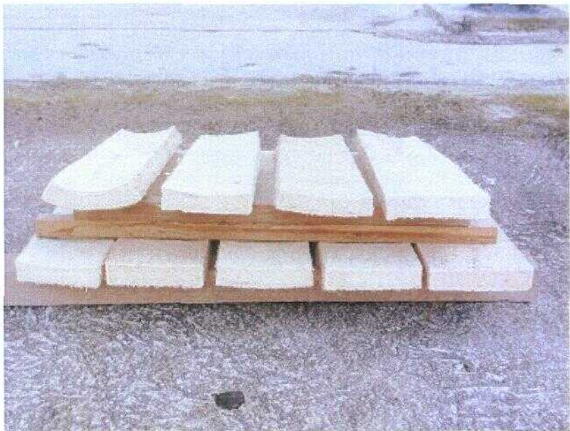
Figure 5 Cupping of the oil palm boards
