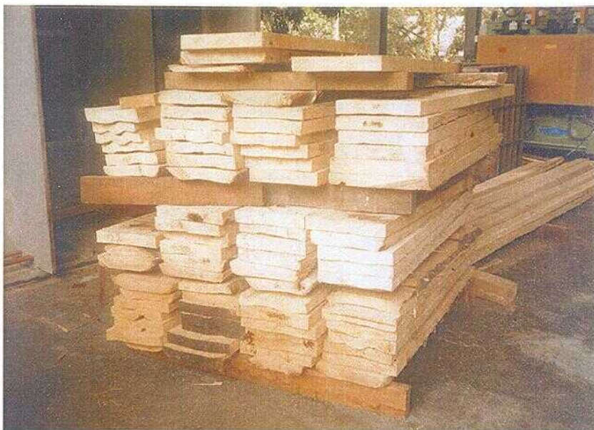
Figure 6 Wavy formation of oil palm boards
