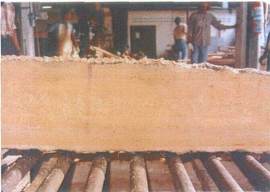
Figure 8 Sawn surface of oil palm board
