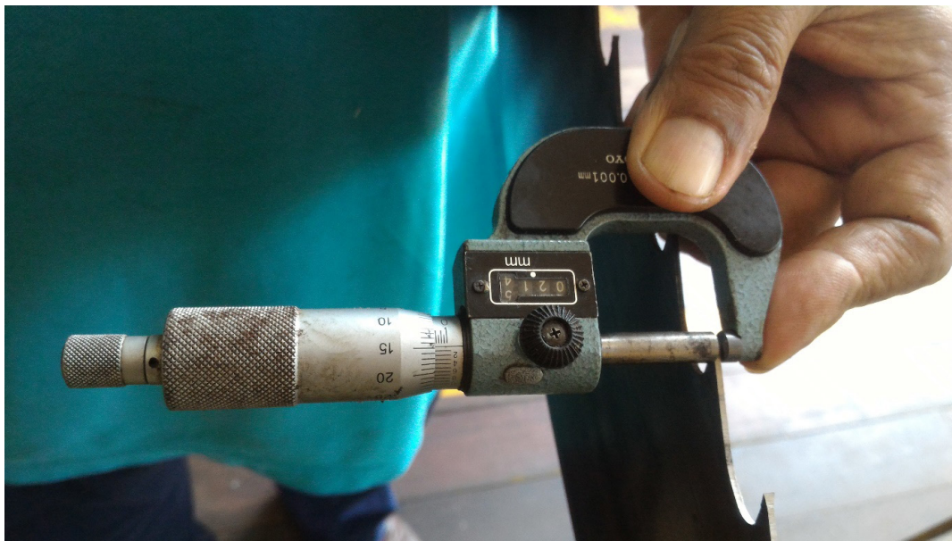
Figure 5 Measuring tooth width using a micrometer
