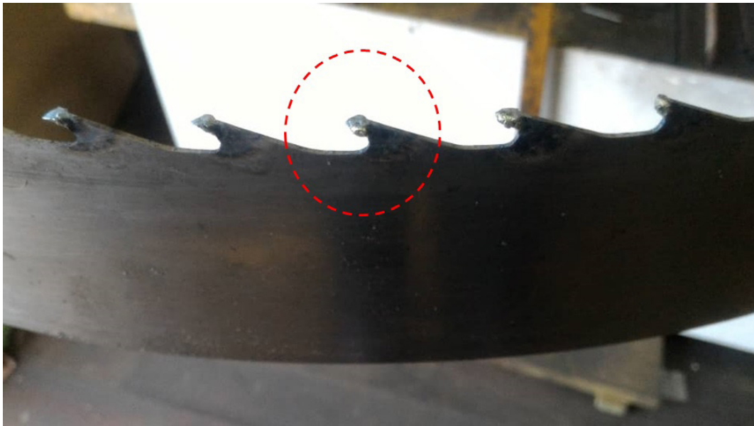
Figure 2 A swaged tooth with stellite tipping before sharpening
