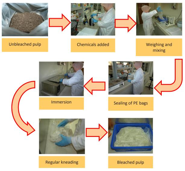
Figure 3 Bleaching process of cellulose
