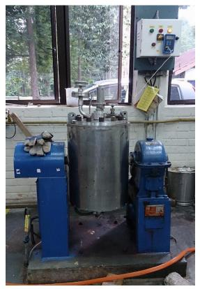
Figure 2 Pulping in 16L rotary digester
