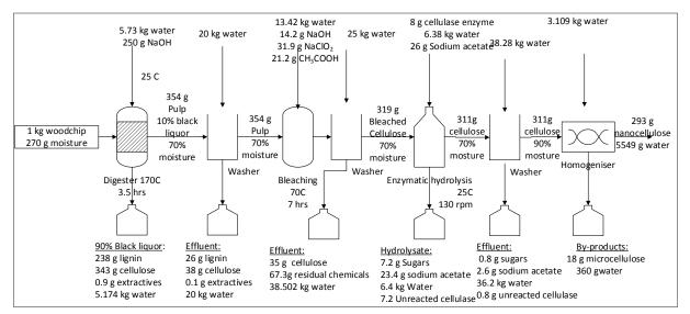
Figure 4 The process for material balance of enzymatic nanocellulose extraction process from *Macaranga tanarius*
