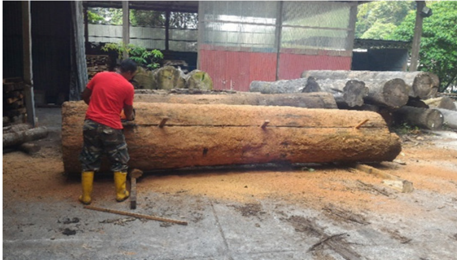
Figure 4 Thin wedges are inserted into saw kerf to maintain the gap for the subsequent sawing
