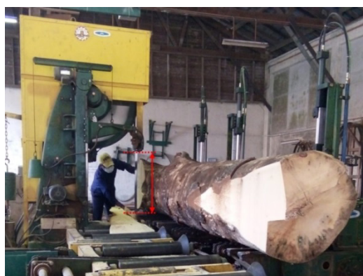
Figure 2 Blade-opening gap of a band saw (red arrow)
