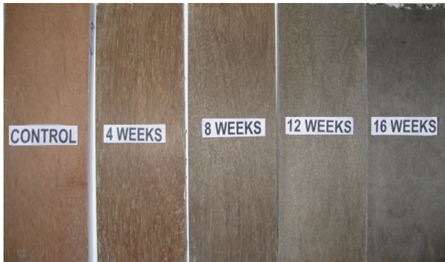
Figure 1 Colour changes for keruing after 16 weeks of exposure to natural weathering
