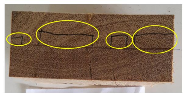
**Figure 2** Poor gluing integrity of a glued-laminated red-balau specimen treated with boron at 6% w/v concentration. The black lines (yellow ellipse) were drawn parallel to the glueline indicating the length of delamination after being subjected to vacuum pressure delamination test.
