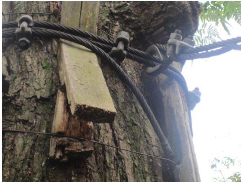
Figure 4 Mechanical failure of a spacer block due to excessive bending load
