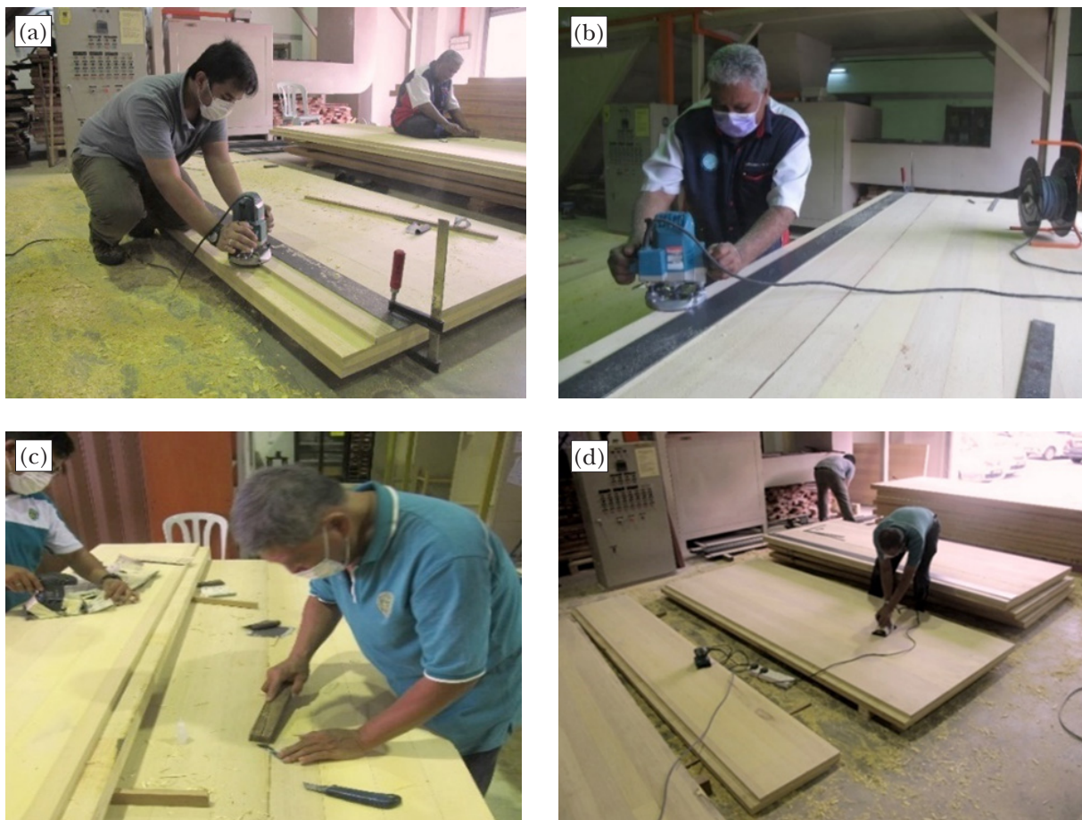
Figure 1 Preparation of the CLT panels, (a) routing of CLT panel for connections, (b) routing work in progress, (c) wood filling and (d) sanding of CLT panel
