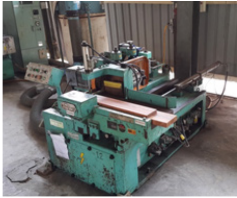
Figure 9 Finger profiler at Wood Lamination Laboratory, FRIM
