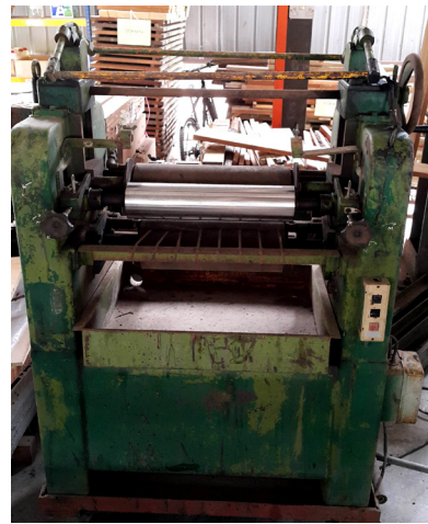
Figure 12 Glue spreaders at Wood Lamination Laboratory, FRIM
