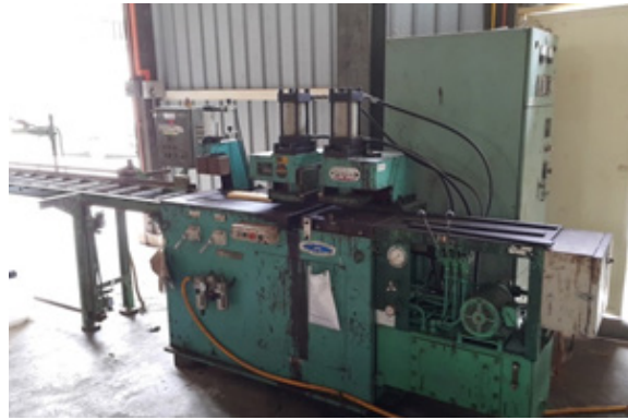
Figure 10 Finger jointer at Wood Lamination Laboratory, FRIM
