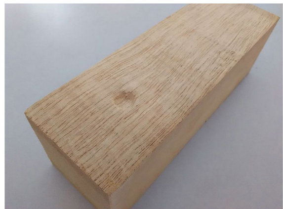
Figure 3 A Janka hardness tested specimen
