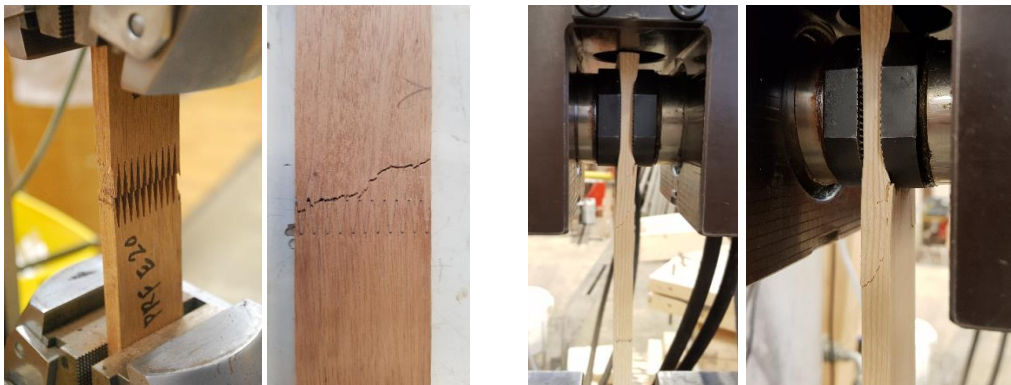
Figure 9 Failure at/near finger joints (left) and crushing at the gripping end section (right)
