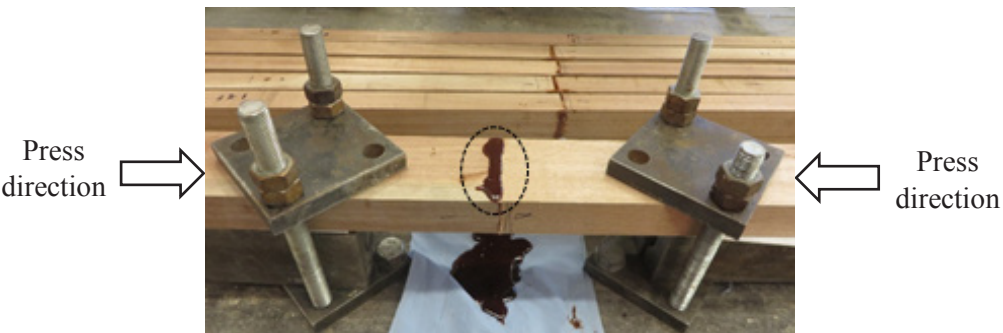
Figure 4 Cramping parallel to grain. Glue squeeze-out (circled)
