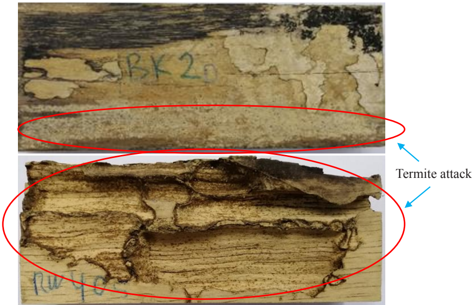
Figure 6 Effects of C. curvignathus infestation on samples of Rhizophora sp. (top) and H. brasiliensis (bottom) after 16 weeks of exposure in above-ground tests
