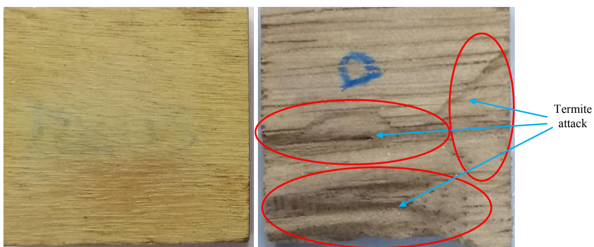
Figure 5 The Rhizophora sp. (left) and H. brasiliensis (right) samples after 28 days' exposure to C. curvignathus
