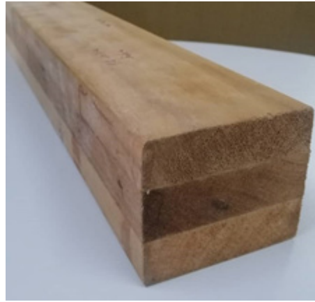
Figure 2 A section of glued-laminated (glulam) timber (Image by Fakrul Hisyam T.)
